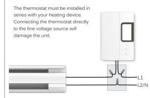
Note: The wires of this thermostat are non-polarized.
