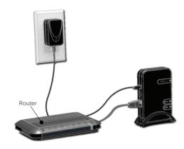
The best diffusion pattern for the internal antenna is reached when the GT125 is installed vertically as shown above.
