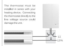
Note: The wires of this thermostat are non-polarized.
