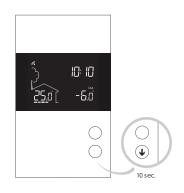
Press the lacksquare and lacksquare buttons simultaneously to save and go to the next parameter. Continue to press until the end of the list to exit the menu.
