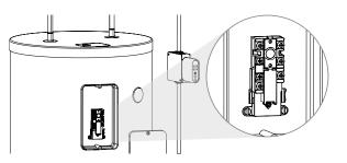
2 Plug the probe into the controller's temperature port.
