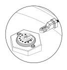
Insert the remote sensor into the R3D remote-ready dial until it snaps into place. Make sure the dial is clean before installing the remote sensor.
