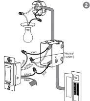
2 Use the provided connectors to connect the wires as follows:
