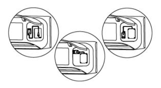
**Note:** The HP6000ZB-GE module wire must be routed through the wire channel; otherwise, the electrical box cover will not close properly.
