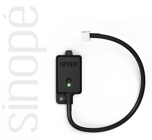
Ductless heat pump interface HP6000ZB-GE
