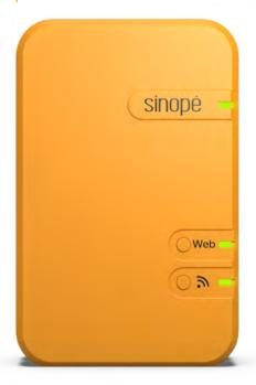
The Sedna Mesh gateway is at the heart of the system's mesh network. It connects the system to the building's Internet connection, transmitting water leak alerts and maintenance notifications to the manager and concerned residents via the Sinopé Smart Systems platform and the Neviweb application.
