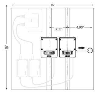
Case 2: Electrical supply on back wall (depth required: minimum 3.17" + depth of electrical outlet), *example with %" NPT ball valve*
