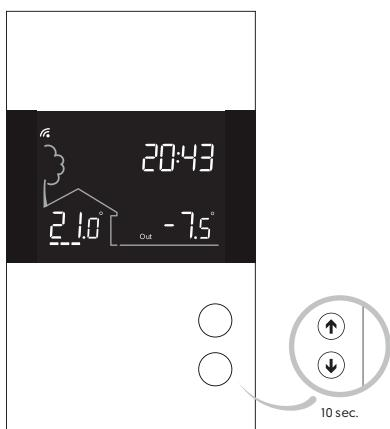
Get the setpoint to its minimum and hold the **↓** button for 10 seconds to access the menu.
