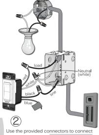
Use the provided connectors to connect the wires as follows: Red —— Load
